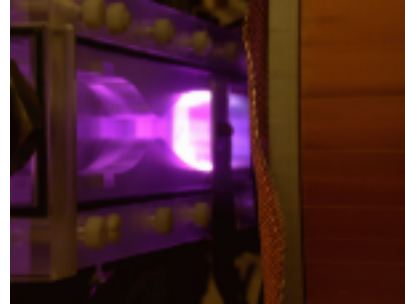
Figure 13 Image of combined RF-DC discharge in B-field, 100 mA DC at 1 Tesla
