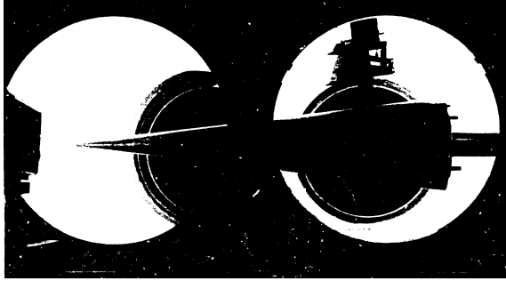
Figure 1. The 7° half-angle blunt cone of Stetson's Mach 7.99 stability experiments (Stetson et al. 1984).
